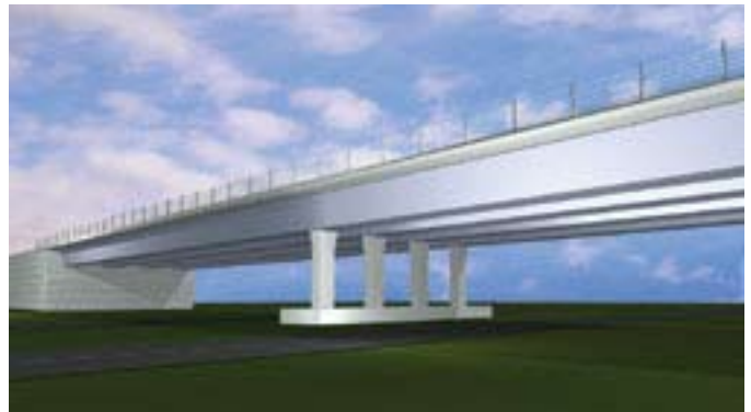
Steel girder design will lighten loads and costs on a new flyover, while clearing space below for Interstate work.
