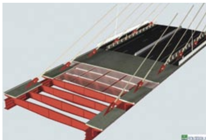
Above: The team pushed the central span length as far as it conceivably could—to go further than 560 m (1,837') would require a steel box girder design for aerodynamic stability.
